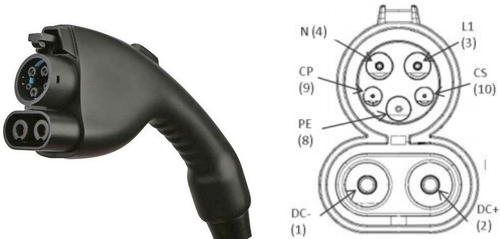
Figure 3.4: Type 1 CCS connector/inlet and pin layout
