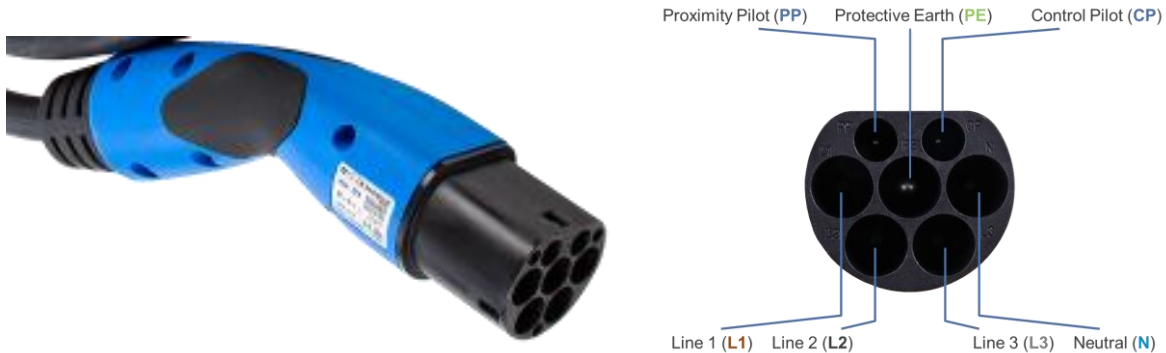
Figure 3.2: Type 2 connector and pin layout
