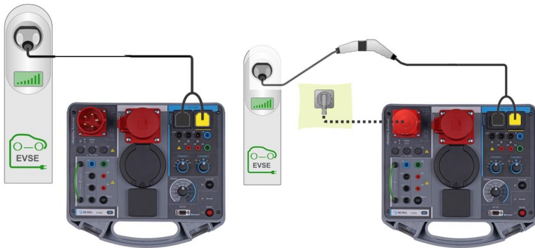
Figure 6.2: 3-Basic EVSE configurations
