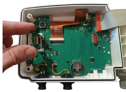
Hold the wireless communication module between your fingers as shown on the picture and slide it between the two holders.
