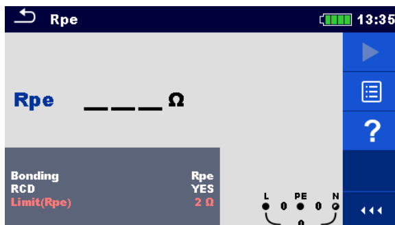
Figure 7.118: PE conductor resistance measurement menu
