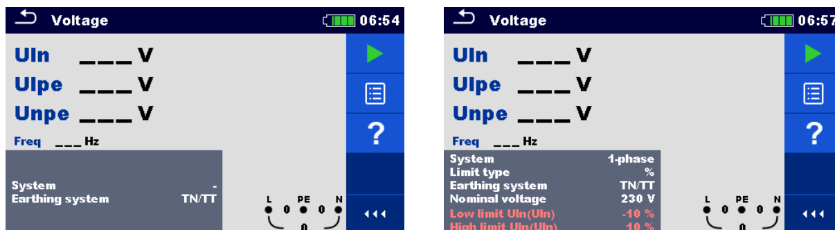
Figure 7.1: Voltage measurement menu
