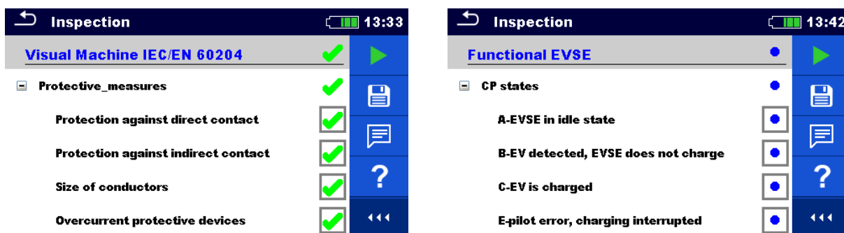
Figure 7.146: Examples of Visual / Functional inspection results
