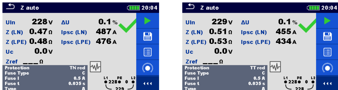
Figure 7.76: Examples of Z auto measurement results
