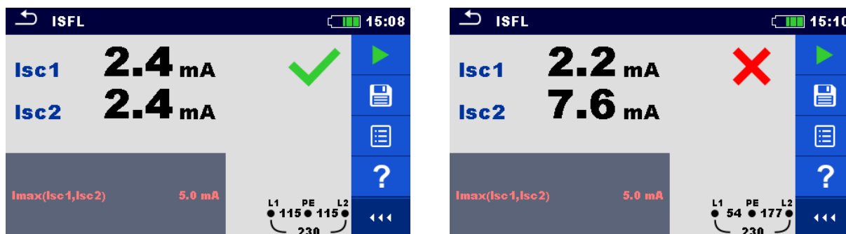
Figure 7.114: Examples of First fault leakage current measurement result
