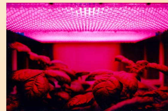
NASA horticulture experiments on potato plants using LED light.
