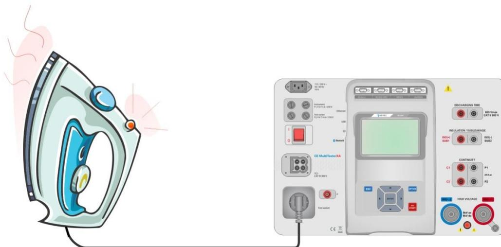
Figure 6.50: Measurement of Ipe Leakage current
