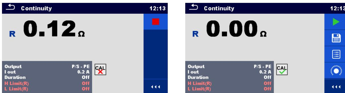
Figure 6.21: Uncompensated and compensated result
