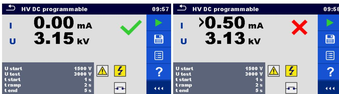
Figure 6.35: Examples of HV DC programmable test results
