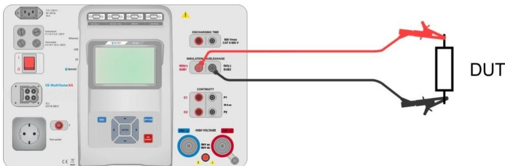
Figure 6.37: Measurement of insulation resistance (ISO(+), ISO(-))
