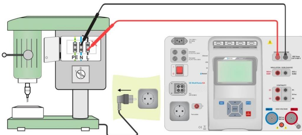
Figure 6.63: Discharging Time test (Output = External)
