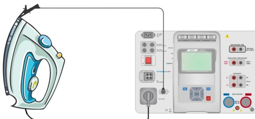
Figure 6.18: Measurement of Continuity P/S - PE
