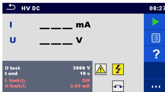
Figure 6.26: HV DC test menu
