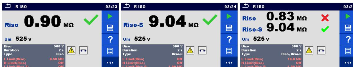
Figure 6.40: Examples of Insulation resistance measurement results
