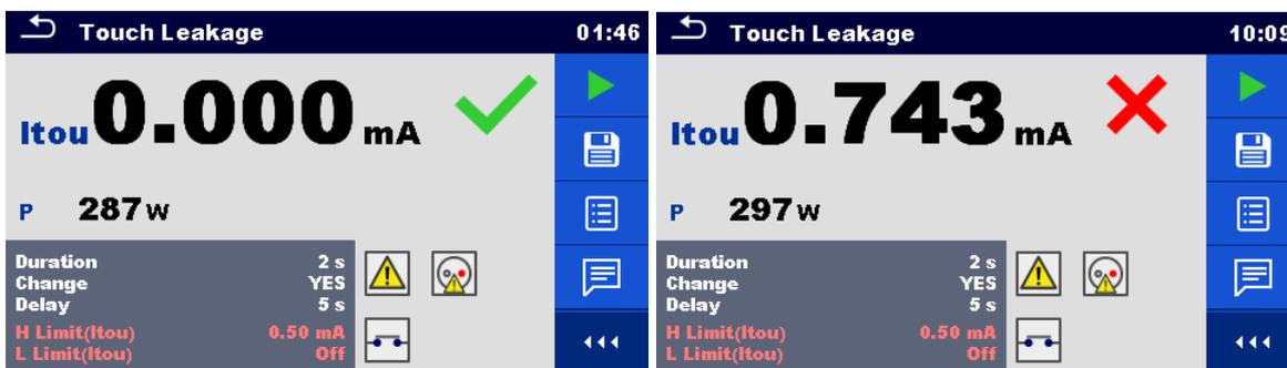
Figure 6.54: Examples of Touch Leakage measurement results
