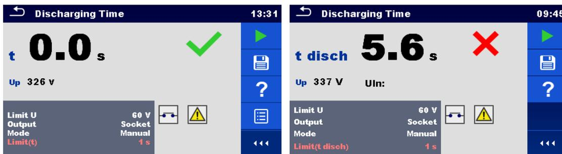
Figure 6.66: Examples of Discharging Time measurement results (Output = Socket)
