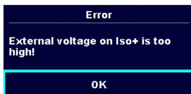
In pre-test a too high external voltage was detected between ISO/SUB and PE terminals. The measurement was cancelled. Press **OK** to continue.
