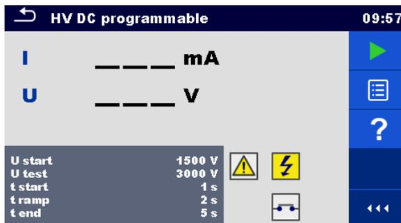
Figure 6.33: HV DC programmable test menu
