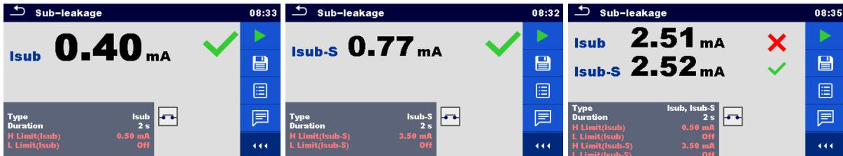
Figure 6.45: Examples of Sub-leakage measurement results
