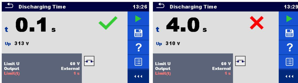
Figure 6.64: Examples of Discharging Time measurement results (Output = External)
