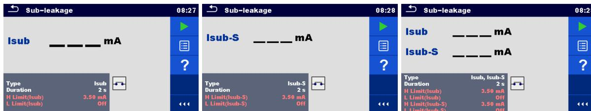
Figure 6.41: Sub Leakage test menus
