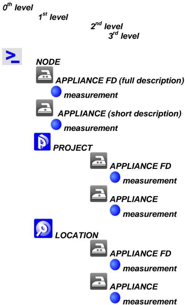
Figure 5.1: Tree structure and its hierarchy
