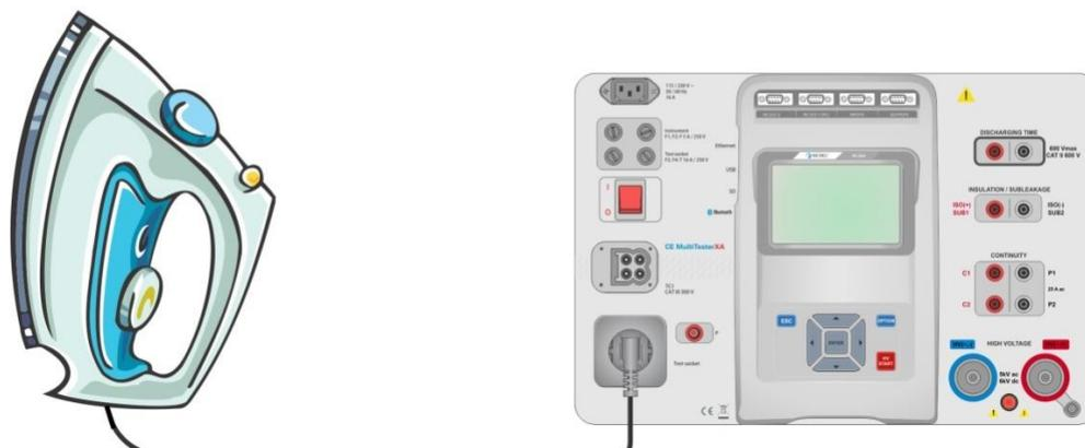
Figure 6.38: Measurement of insulation resistance (Socket LN - PE)
