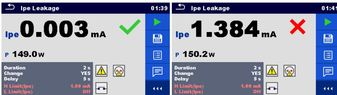
Figure 6.51: Examples of Ipe Leakage measurement results
