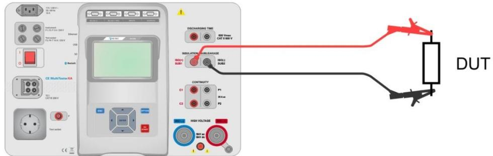
Figure 6.42: Measurement of Sub-leakage (SUB1, SUB2)
