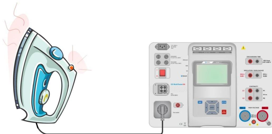
Figure 6.47: Measurement of Differential Leakage current
