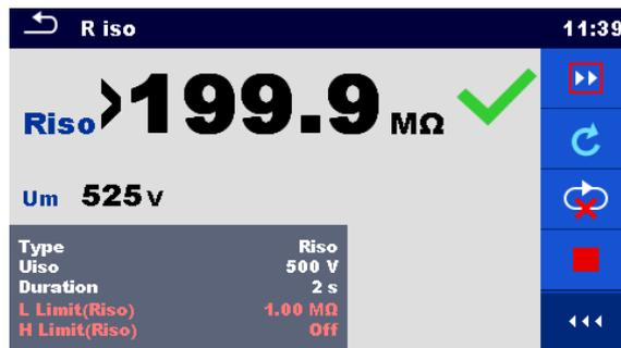
Figure 7.8: Auto Sequence® – example of a finished measurement with options for proceeding
