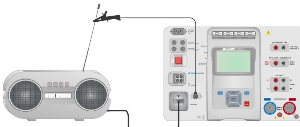
Figure 6.39: Measurement of Riso, Riso-S (socket)
