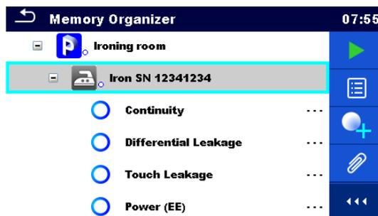
Figure 5.4: Example of status - No measurement result(s)
