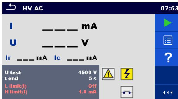
Figure 6.23: HV AC test menu
