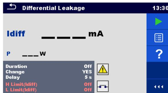
Figure 6.46: Differential Leakage test menu
