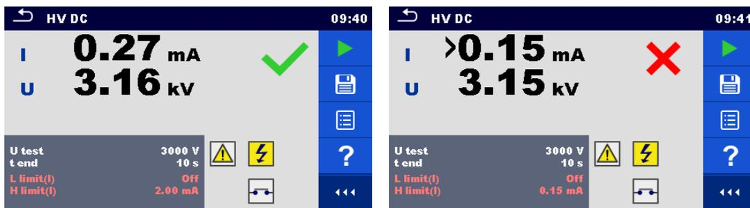
Figure 6.28: Examples of HV DC measurement results
