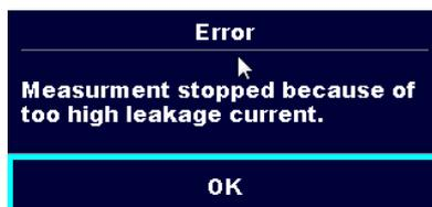
The measured leakage ( $I_{\text{diff}}$ ,  $I_{\text{pe}}$ ,  $I_{\text{touch}}$ ) current was higher than 20 mA. Measurement was aborted. Press **OK** to continue.
