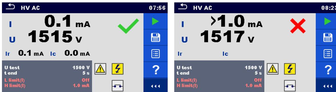
Figure 6.25: Examples of HV AC measurement results
