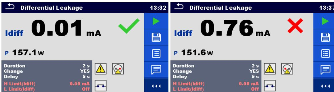
Figure 6.48: Examples of Differential Leakage measurement results
