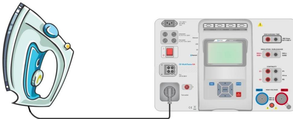
Figure 6.43: Measurement of Sub-leakage (socket LN-PE)
