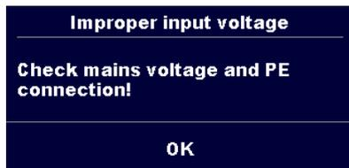
Warning for improper supply voltage condition. If pressing **OK** instrument will continue to work in a limited mode (measurements are disabled).
