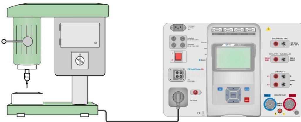
Figure 6.65: Discharging Time test (Output = Socket)
