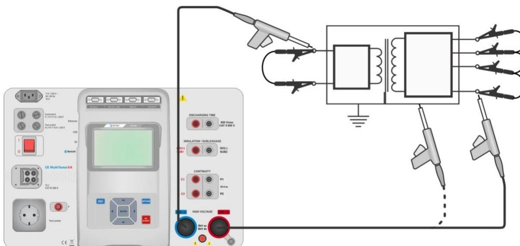
Figure 6.24: HV AC measurement
