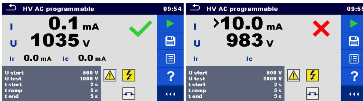
Figure 6.32: Examples of HV AC programmable test results
