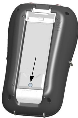
Figure 7.2: Closing the battery compartment cover
