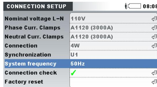
Figure 4.2: Connection setup menu
