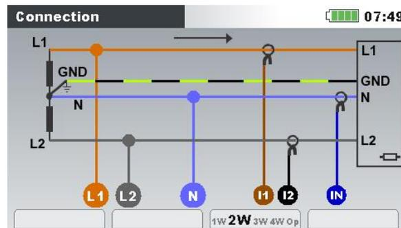
Figure 4.11: Choosing 2-phase 4-wire system on instrument
