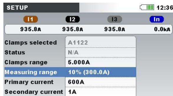
Figure 4.17: Selecting 10% of current clamps range
