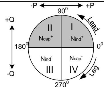
and plus sign indicates consumed fundamental reactive power. This parameter is recorded separately for each quadrant as shown on figure. See 5.1.5 for definition.
