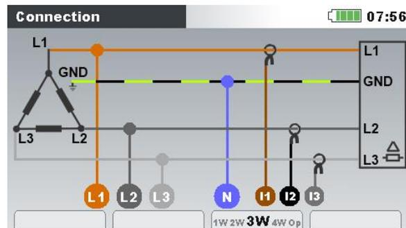
Figure 4.5: Choosing 3-phase 3-wire system on instrument
