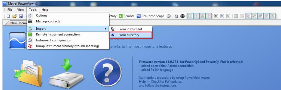
Alternatively user can Import data directly from instrument and use USB connection
