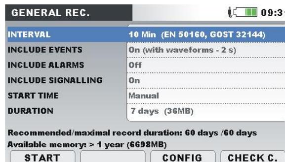
Figure 3.46: General recorder setup screen
