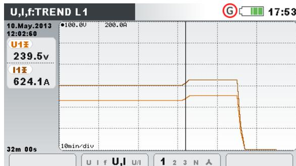
Figure 3.18: Voltage and current trend (single mode)
