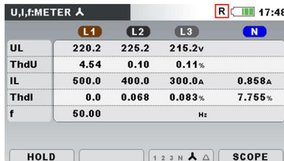
Figure 3.56: U,i,f meter screen in recalled snapshot record
