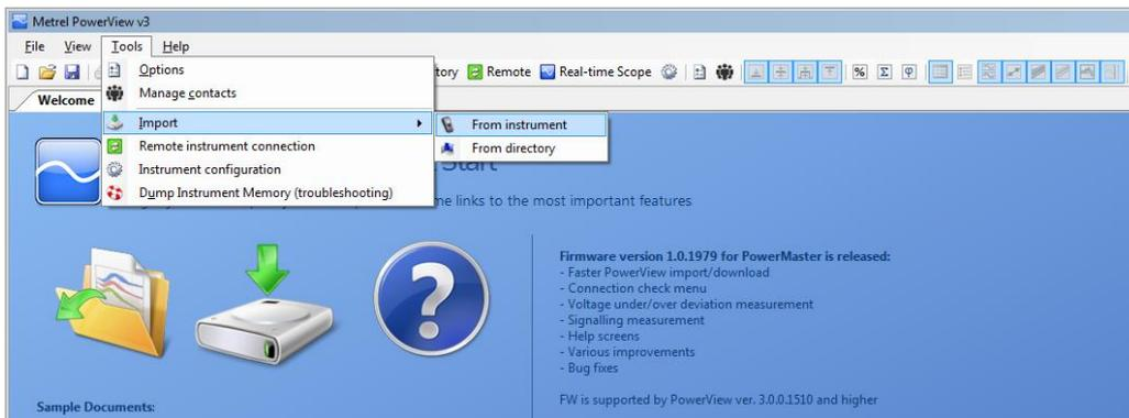
Download window will be displayed, and PowerView v3.0 will immediately try to connect to the instrument and detect the instrument model and firmware version.
