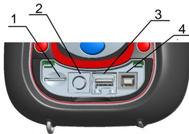
Figure 2.3: Side connector panel
