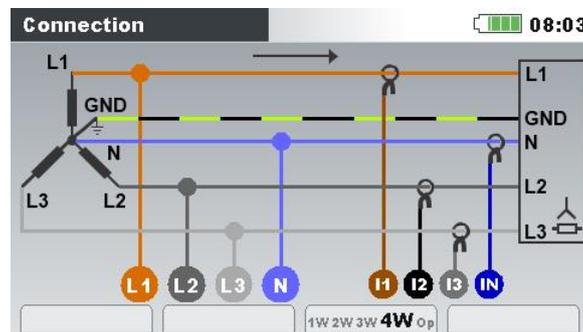
Figure 4.3: Choosing 3-phase 4-wire system on instrument
