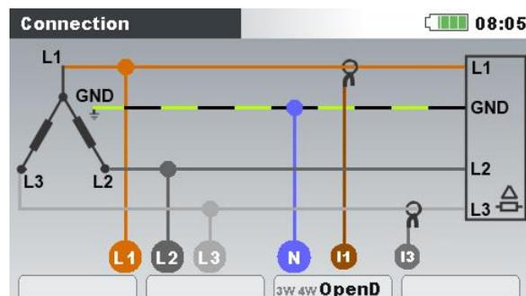
Figure 4.7: Choosing Open Delta (Aaron) 3-wire system on instrument
