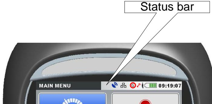
Figure 3.3: Instrument status bar
