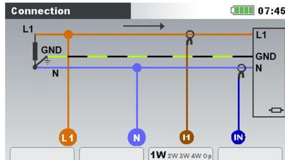
Figure 4.9: Choosing 1-phase 3-wire system on instrument
