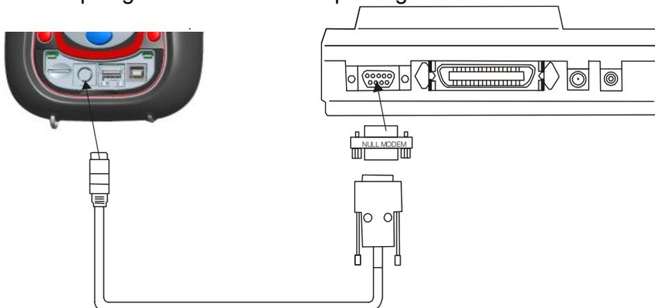
Figure 4.20: Connecting printer DPU 414 with instrument
