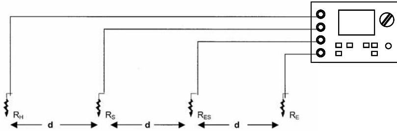
The ground resistivity is calculated by the Wenner method using the following formula :
