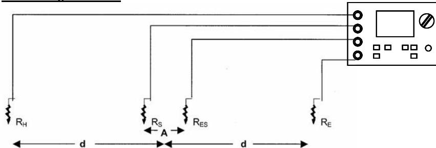
The ground resistivity is calculated by the Schlumberger method using the following formula:
