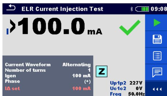
Figure 7.114: Example of ELR Current Injection Test measurement result
