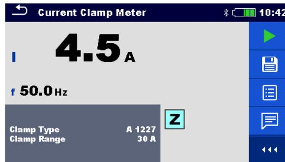
Figure 7.80: Example of Current Clamp Meter measurement result
