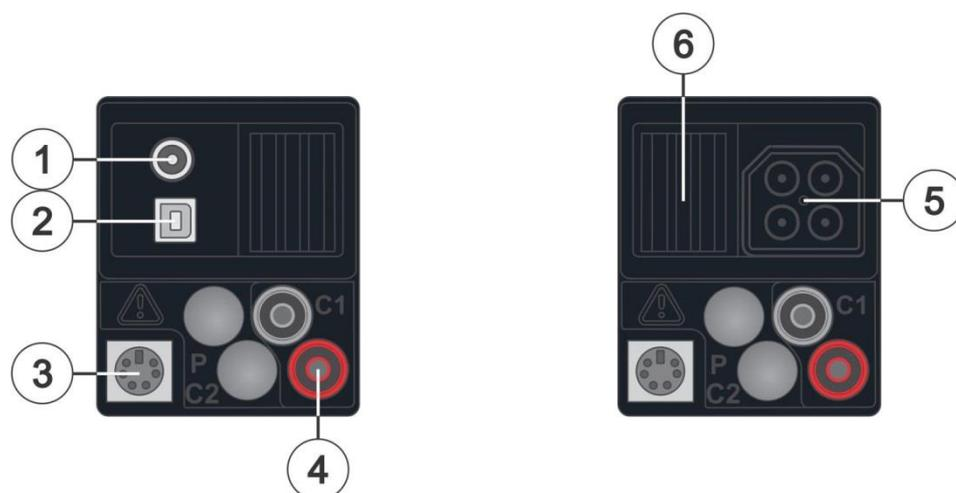
Figure 3.2: Connector panel
