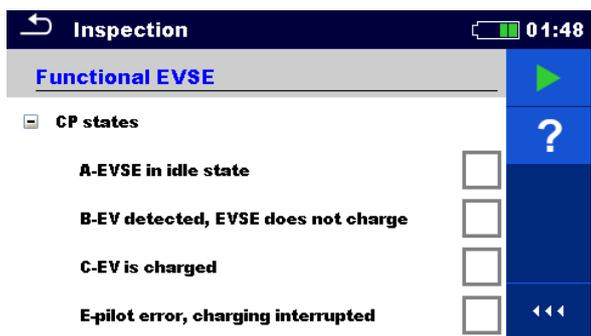
Figure 7.126: Example of Functional inspection menu
