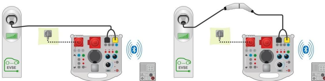
Figure 7.118: Diagnostic Test, EV simulator and Errors sub-tests - connection to EVSE
