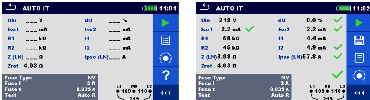
Figure 7.105: Examples of AUTO IT measurement results
