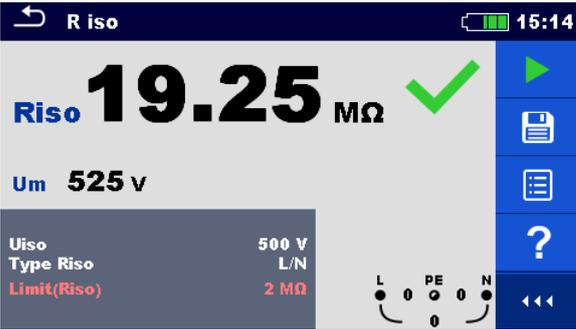
Results / sub-results after re-run of recalled measurement.
