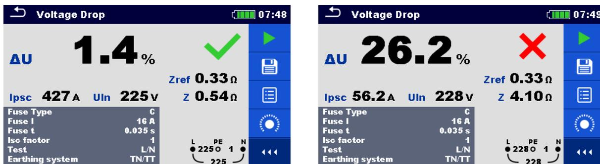
Figure 7.55: Examples of Voltage drop measurement result (STEP 2)
