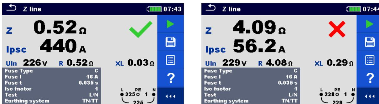
**Figure 7.45: Examples of Line impedance measurement result**
