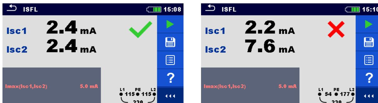
Figure 7.84: Examples of First fault leakage current measurement result
