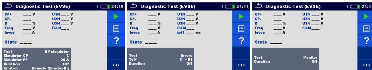
Figure 7.117: Diagnostic Test (EVSE) start screens – EV simulator, Errors and Monitor
