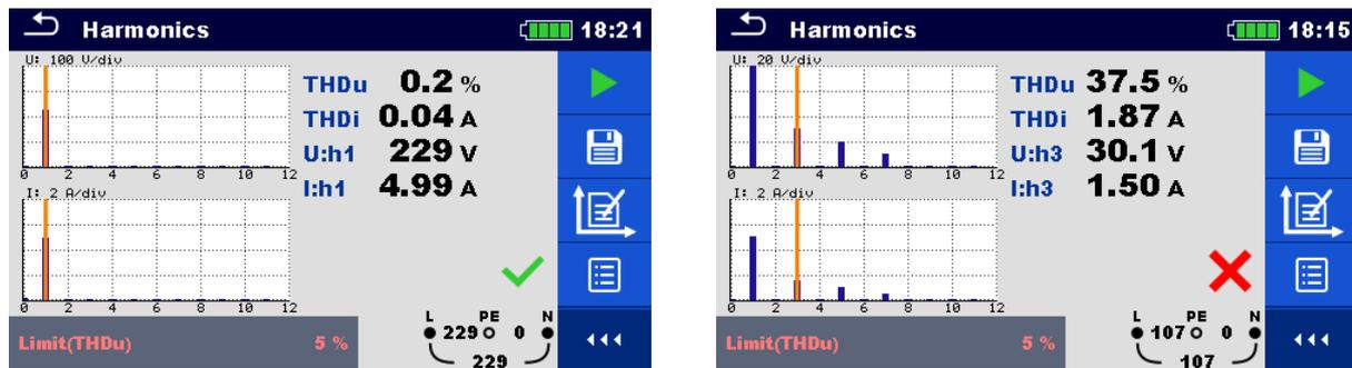
Figure 7.74: Examples of Harmonics measurement results
