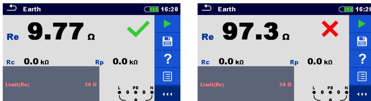
Figure 7.62: Examples of Earth resistance measurement result
