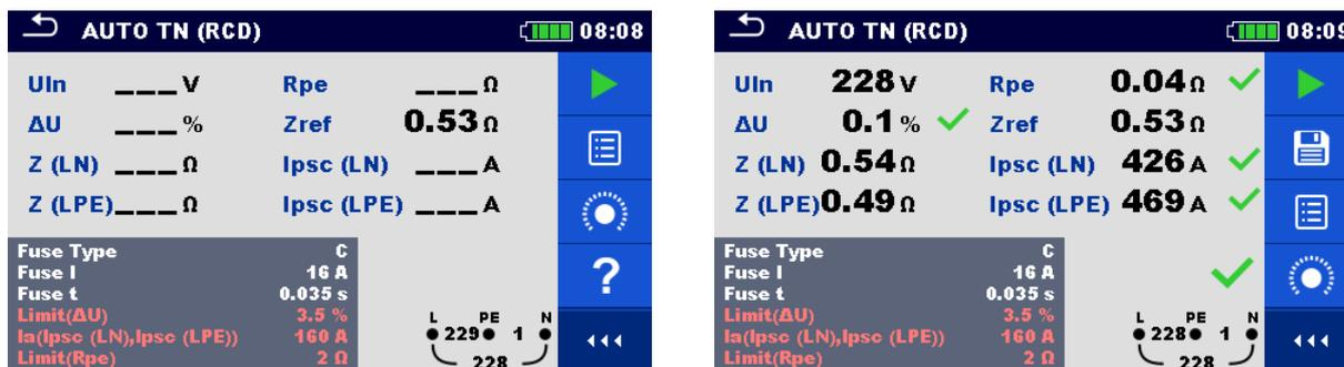
Figure 7.99: Examples of AUTO TN (RCD) measurement results
