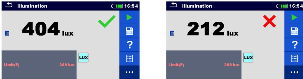
Figure 7.93: Examples of Illumination measurement result
