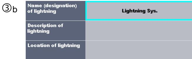
In menu for editing name and parameters the parameter's value can be selected from a dropdown list or entered via keypad. Refer to chapter **4 Instrument operation** for more information about keypad operation..
