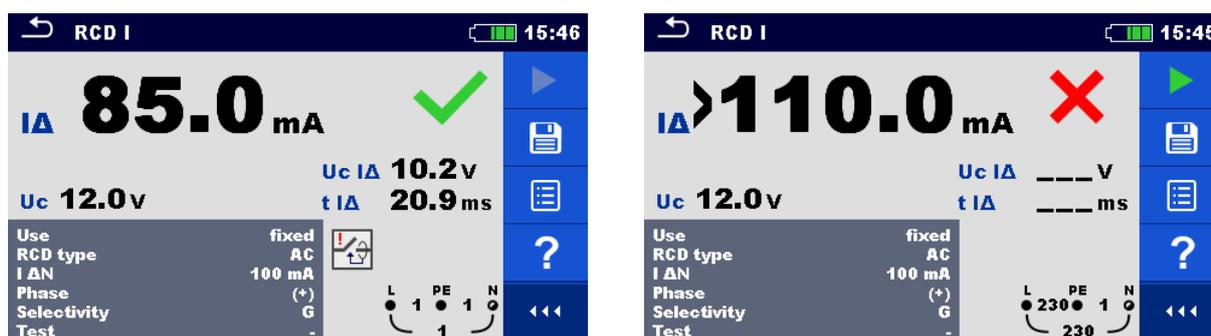
Figure 7.31: Examples of Trip-out current measurement result
