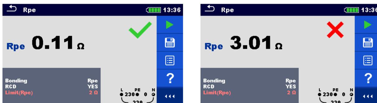
Figure 7.90: Examples of PE conductor resistance measurement result
