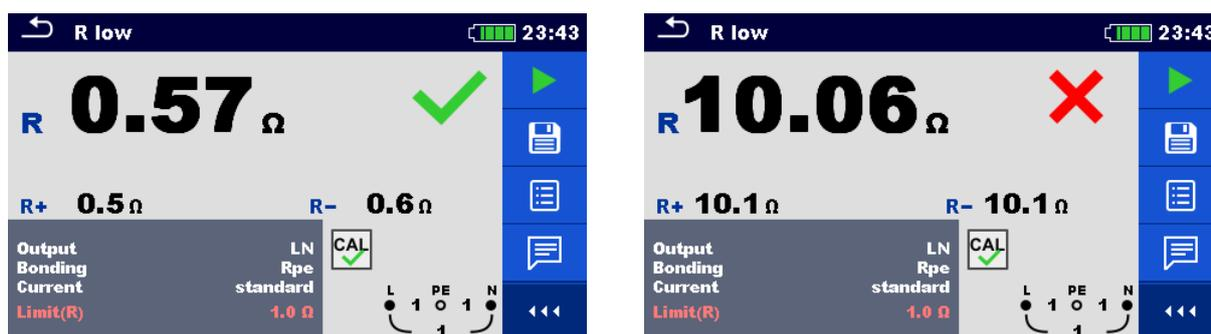
Figure 7.21: Examples of R low measurement result
