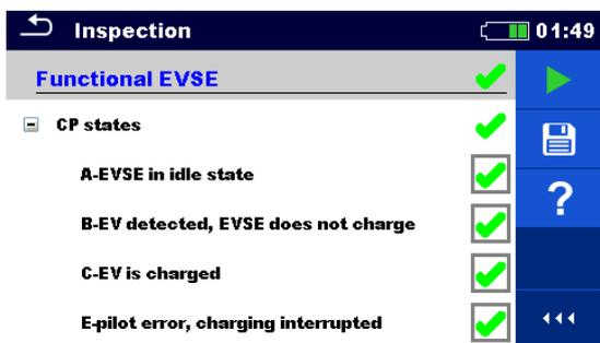
Figure 7.128: Example of Functional inspection results
