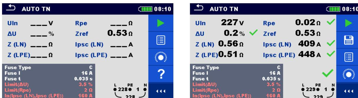
Figure 7.102: Examples of AUTO TN measurement results
