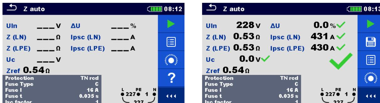
Figure 7.108: Example of Z auto measurement results
