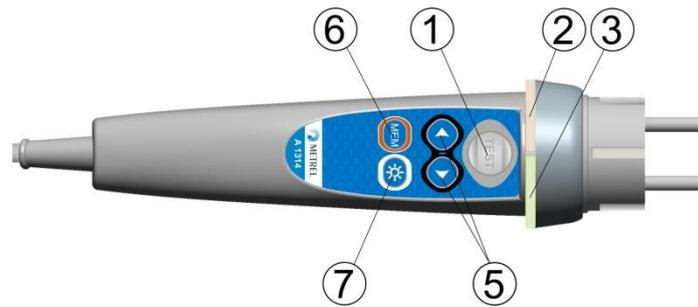
Figure B.2: Front side Plug commander (A 1314)
