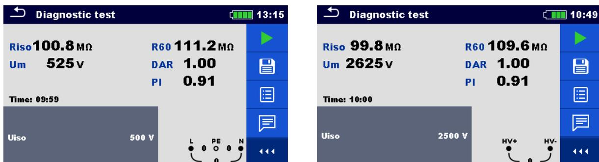
Figure 7.14: Examples of Diagnostic test result
