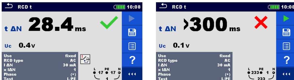
Figure 7.30: Examples of Trip-out time measurement result
