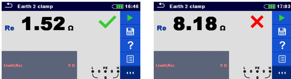
Figure 7.65: Examples of Contactless earthing resistance measurement result
