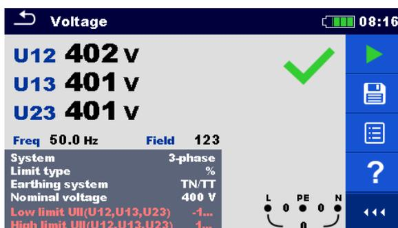
Figure 7.5: Examples of Voltage measurement in three-phase system
