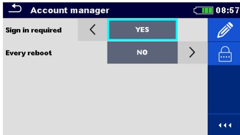
Field for setting if signing in is required to work with the instrument.
