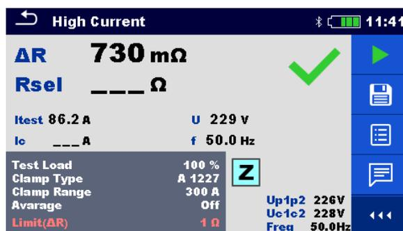
Figure 7.51: Example of High Current measurement result
