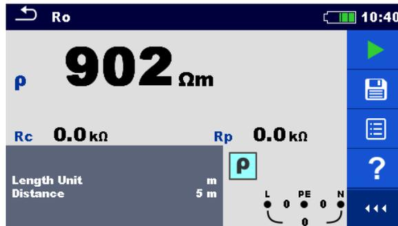
Figure 7.68: Example of Specific earth resistance measurement result
