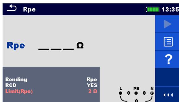
Figure 7.88: PE conductor resistance measurement menu
