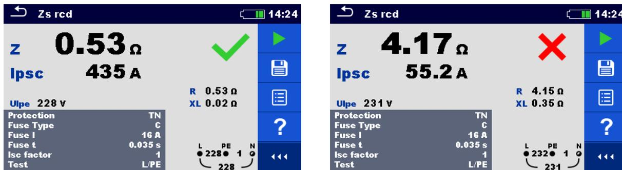
Figure 7.38: Examples of Zs rcd measurement result
