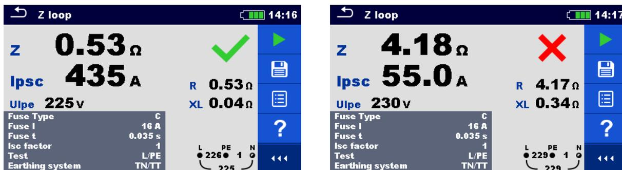
**Figure 7.35: Examples of Loop impedance measurement result**
