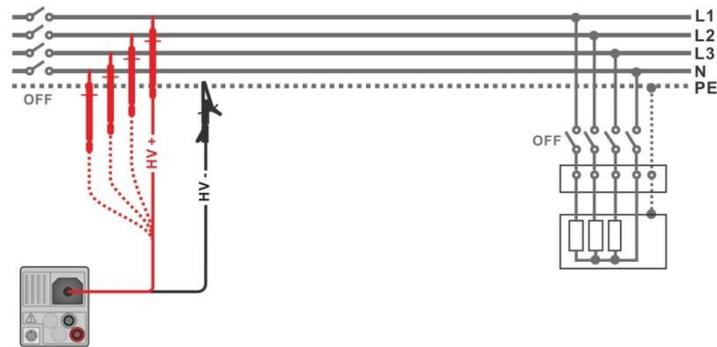
Figure 7.13: Connection of 2.5 kV test lead ( $U_N = 2.5 \text{ kV}$ )
