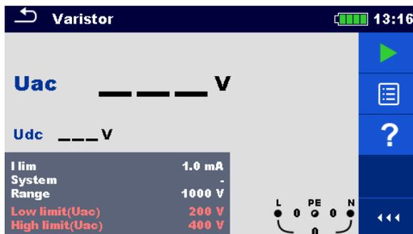
Figure 7.15: Varistor test main menu
