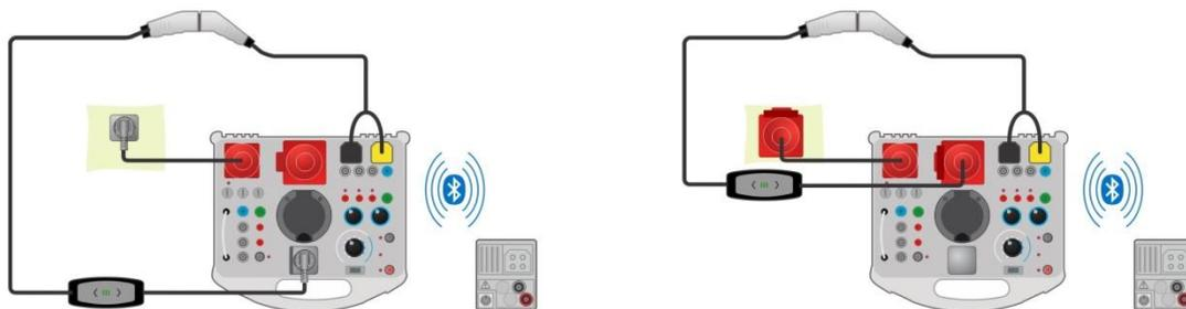
Figure 7.119: Diagnostic Test, EV simulator and Errors sub-tests - connection to Mode 2 charging cable powered from Analyser
