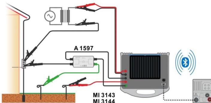
Figure 7.57: Touch voltage measurement – Connection of MI 3143 or MI 3144
