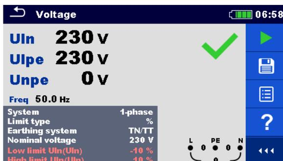
Figure 7.4: Example of Voltage measurement in single-phase system
