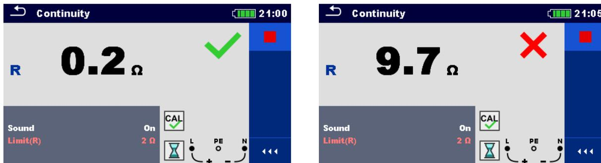
Figure 7.24: Examples of Continuity resistance measurement result
