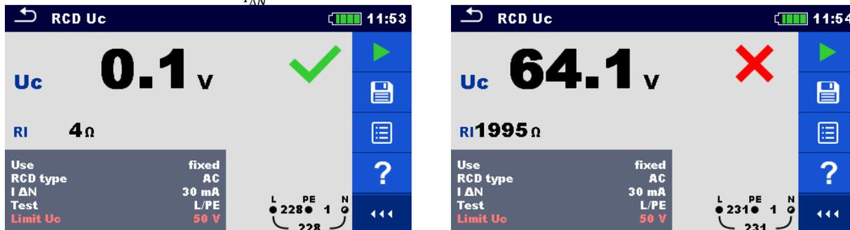
Figure 7.29: Examples of Contact voltage measurement result
