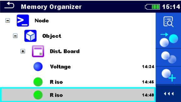
Retested measurement is saved under same structure object as original one.
