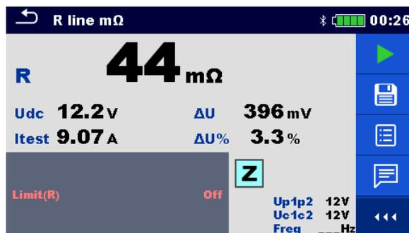
Figure 7.111: Example of R line mΩ measurement result
