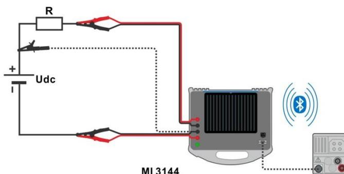
Figure 7.110: R line mΩ measurement connection
