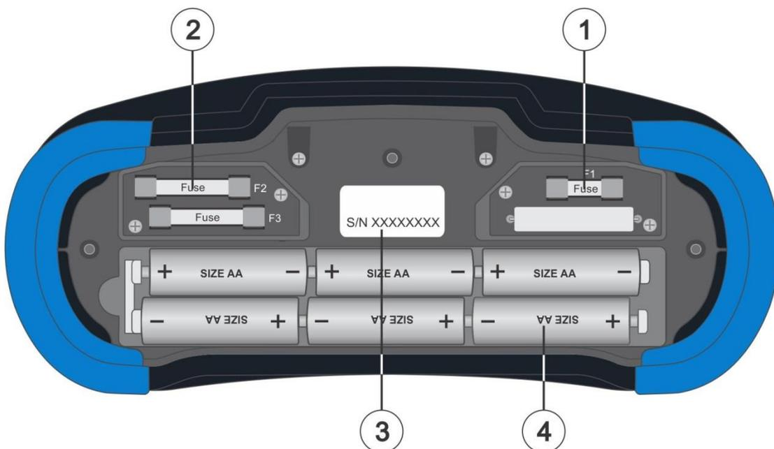
Figure 3.4: Battery and fuse compartment
